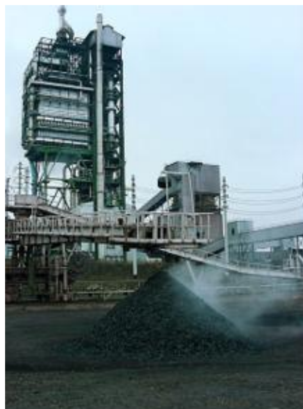
FIGURE 10: MINOR VAPOUR PLUME AS HOT MATERIAL MEETS ATMOSPHERIC MOISTURE Image courtesy of Energiron
