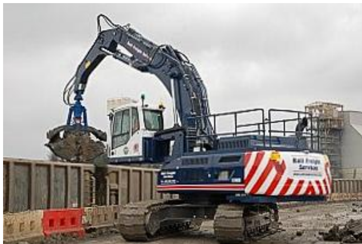
FIGURE 6: RAILCAR LOADERS HAVING “SOFT-LOADING” CAPABILITY (TO MINIMISE DROP HEIGHT) Images sourced from: left - Hub-4.com; right - PiercePacific.com
