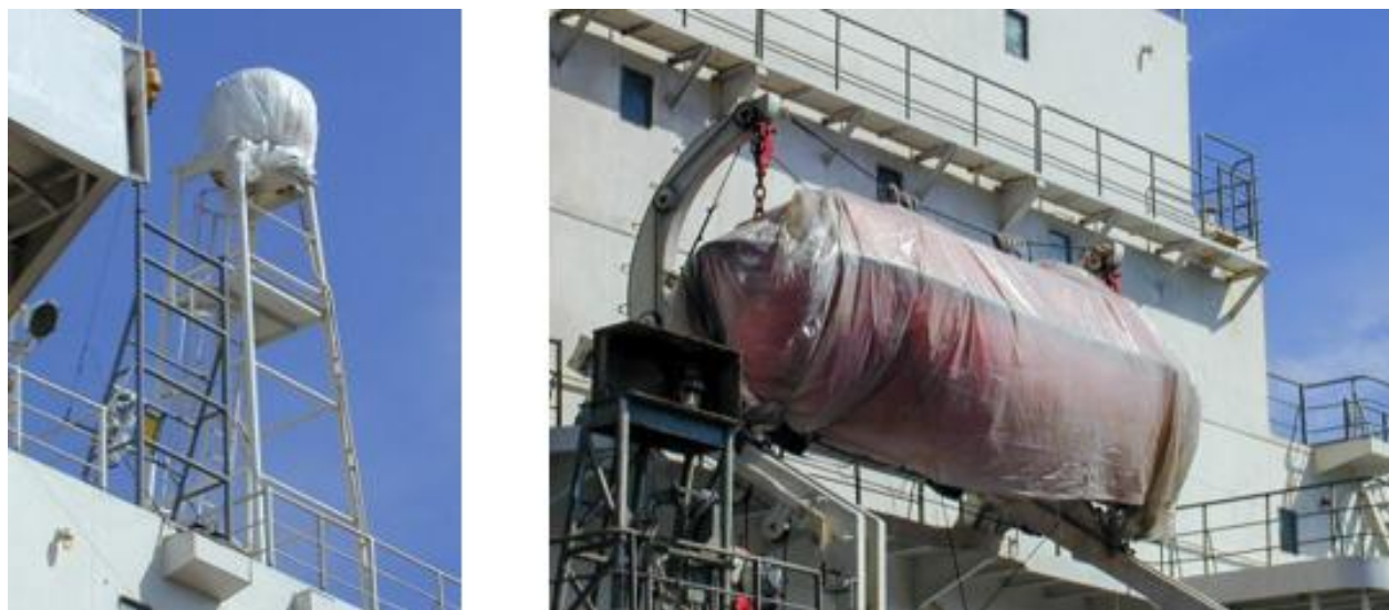
FIGURE 16: PROTECTING VESSEL EQUIPMENT FROM DRI DUST
