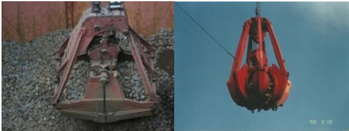
FIGURE 20: CLAM SHELL GRAB FOR SMALLER INGOTS/PIECES (LEFT) AND ORANGE PEEL GRAPPLE FOR LARGER INGOTS/PIECES (RIGHT)
