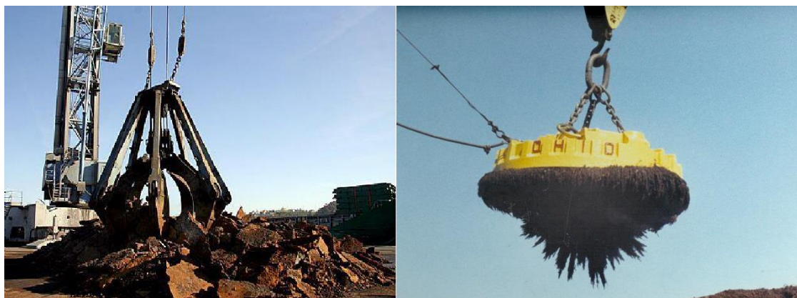
FIGURE 7: GRAB AND MAGNET FOR HANDLING SCRAP PIG IRON
