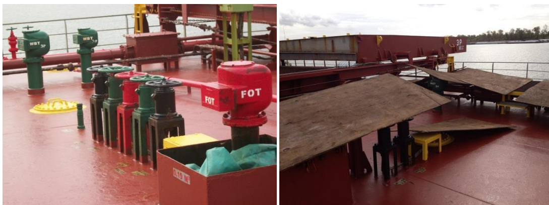
FIGURE 21: EXPOSED ABOVE DECK PIPING/VALVES (LEFT) AND PLYWOOD USED TO PROTECT ABOVE DECK PIPING AND VALVES (RIGHT)
