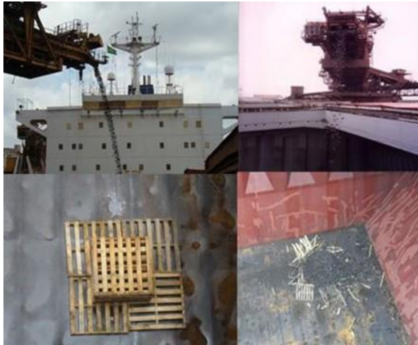
FIGURE 10: USE OF PALLETS TO ABSORB THE IMPACT OF FALLING INGOTS
