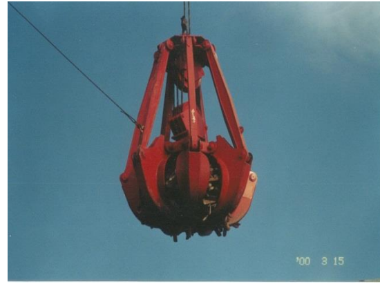
Figure 18 - Clam shell grab for small pig iron (left) and orange peel grapple for large pig iron (right)
