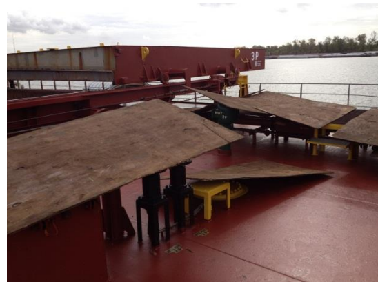
Figure 19 - Exposed above deck piping and valves (left) and plywood used to protect above deck piping and valves (right)
