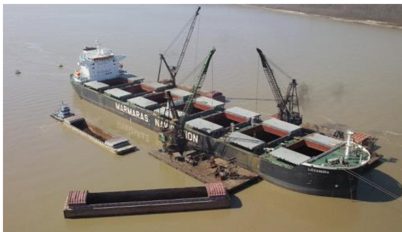
Figure 15 - Vessels anchored mid-stream and secured to mid-stream buoys, floating cranes secured alongside the vessel
