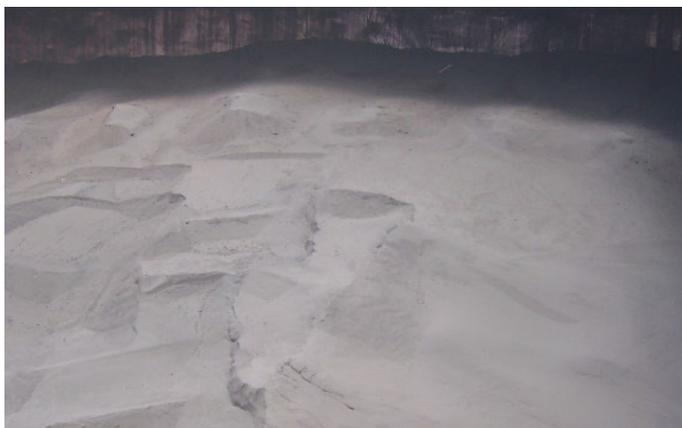
**DRI (C):** a porous, black/grey metallic material generated as a by-product of the manufacturing and handling processes of DRI (A) and/or DRI (B). The density of DRI (C) is less than 5,000 kg/m<sup>3</sup>. A loading requirement for DRI (C) is that the moisture content must be maximum 0.3%.
