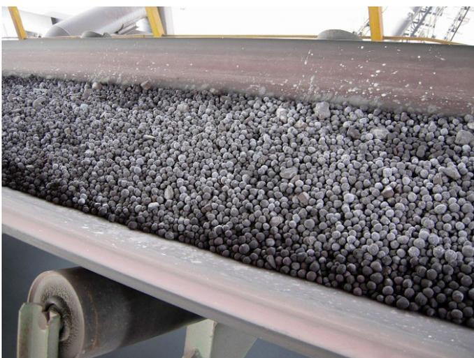
**DRI (B):** a highly porous, black/grey metallic material formed by the reduction (removal of oxygen) of iron oxide at temperatures below the fusion point of iron. Cold-moulded briquettes are defined as those which have been moulded at a temperature less than 650°C or which have a density of less than 5,000 kg/m<sup>3</sup>. Fines and small particles under 6.35 mm in size shall not exceed 5% by weight.
