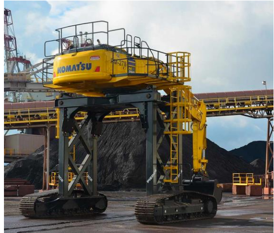
Figure 6: Railcar loaders having “soft-loading” capability (to minimise drop height)
