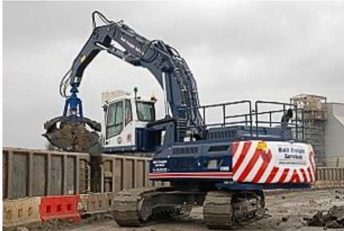
Figure 6: Railcar loaders having “soft-loading” capability (to minimise drop height)
