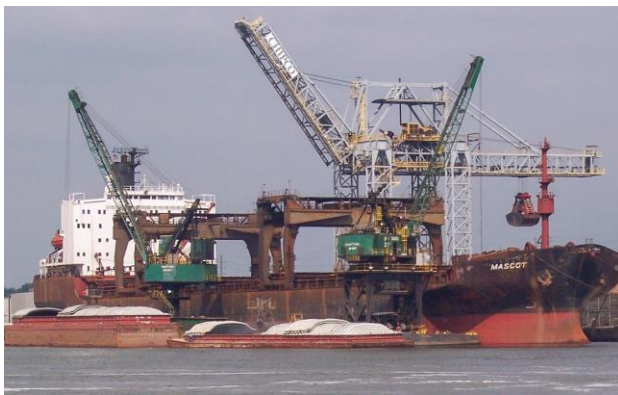
Figure 15: Simultaneous transfer to barges and port storage using vessel floating cranes
