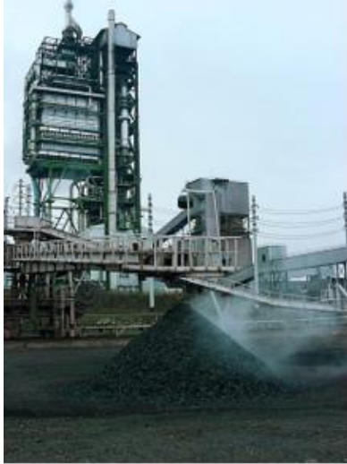
Figure 10: Minor vapour plume as hot material meets atmospheric moisture
