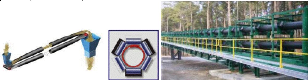
Figure 8: Pipe conveyor schematic and example system
