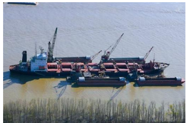
Figure 16: Midstreaming: discharging cargo to barges using floating cranes on both sides of the vessel
