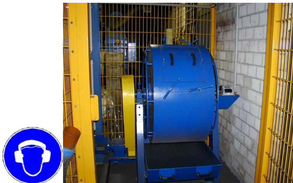
Figure 6: The tumble drum for determination of the tumble and abrasion index (ear protection required!)
