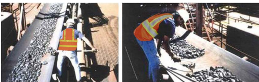
Figure 1: Surveyors collecting increments using “stopped belt sampling” (images courtesy of Marine Inspection, LLC)
