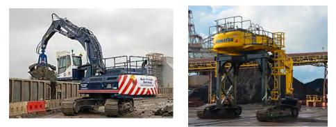
Figure 6: Railcar loaders having "soft-loading" capability (to minimise drop height) (Images sourced from: left - Hub-4.com; right - PiercePacific.com)
