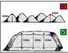
Figure 9: Proper stacking of HBI (Diagram courtesy of BHP)
