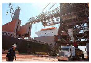
Figure 24: Transfer from hopper to truck (Photo courtesy of Port of Corpus Christi, TX)
