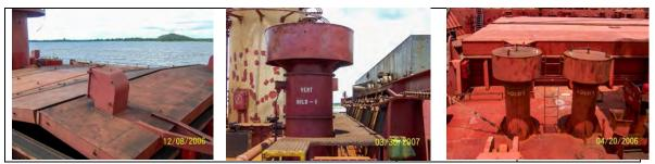
Figure 16: Photo collage of typical ventilators on hatch covers Left: single natural gravity vent Centre: single mushroom style fan-assisted vent Right: dual mushroom style fan-assisted (Images courtesy of IIMA)
