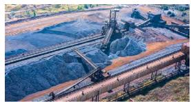
Figure 4: Travelling conveyor-stacker and bucket wheel reclaimer at HBI Plant yard (Image courtesy of Metalloinvest)
