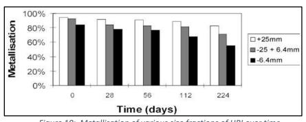
Figure 10: Metallisation of various size fractions of HBI over time (samples from stockpile outer layer) (Chart courtesy of BHP)
