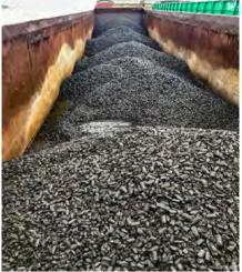
Figure 22: Correct loading of HBI to barges (Diagram courtesy of BHP, imageo courtesy of Marine Inspection)
