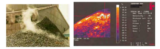
Figure 13: HBI pile self-heating incident, with thermal profile (Images courtesy of BHP)
