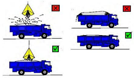
Figure 25: Keep drop heights low and avoid overloading railcars and trucks (Diagrams courtesy of BHP)
