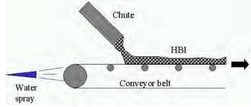
Figure 15: Illustration of use of water spray to suppress dust (Diagram courtesy of BHP)
