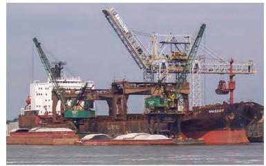
Figure 19: Simultaneous transfer to barges and port storage using vessel floating cranes (Image courtesy of Marine Inspection, LLC)
