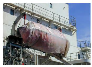
Figure 21: Protecting vessel equipment from HBI dust (Images courtesy of Mascinenfabrik Köppern)
