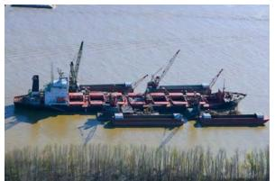
Figure 20: "Midstreaming": discharging cargo to barges using floating cranes on both sides of the vessel (Image courtesy of CBG)
