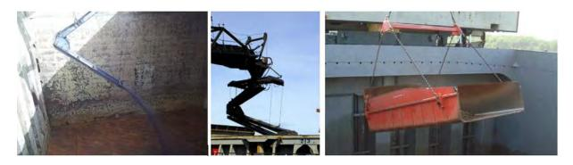
Figure 17: Photos of "soft-loading" devices
