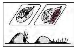
Figure 14: Controlling hot spots in an HBI pile Top: View from overhead; Left: >100°C (212°F) hot spot identified, Right: HBI spread out to dissipate heat build-up (Diagram courtesy of BHP)
