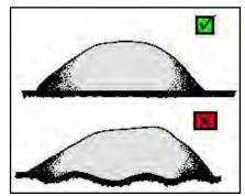
Figure 8: Correct storage base for HBI (Diagram courtesy of BHP)
