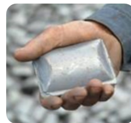
Hot Briquetted Iron
