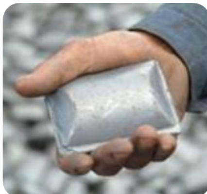
Hot Briquetted Iron
